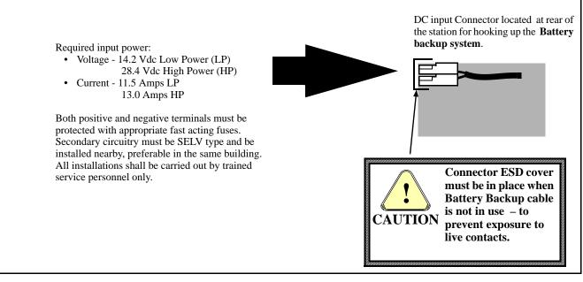
Figure 10. Making Connections to Storage Battery
