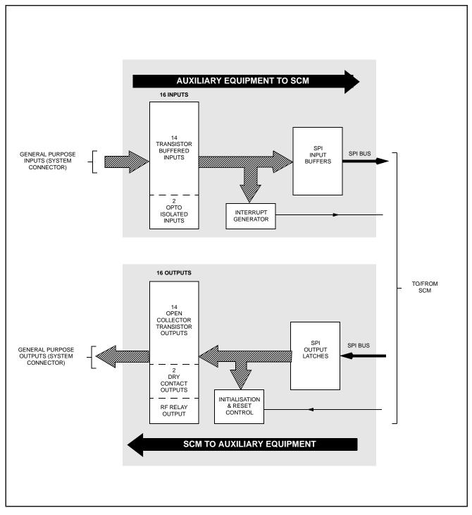
Figure 3. CLN1206 – Auxiliary I/O Board Functional Block Diagram
