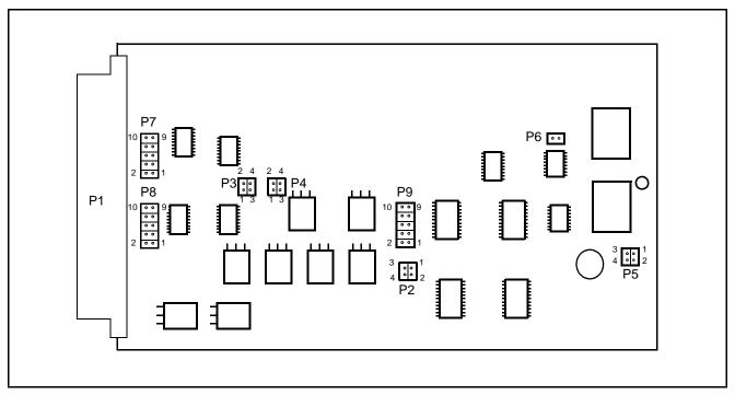
Figure 2. CLN1206 Auxiliary I/O Board Jumpers
