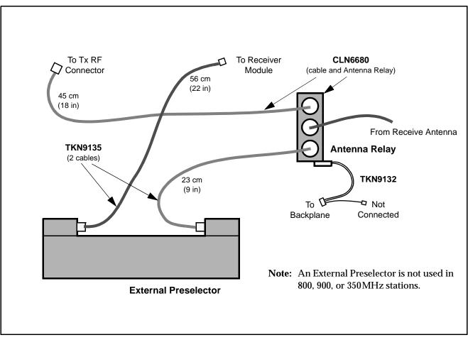
Figure 3. Antenna Relay and External Preselector - Cable Kits
