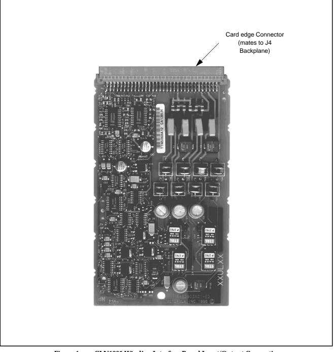
Figure 1. CLN1205 Wireline Interface Board Input/Output Connections
