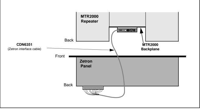
Figure 2. MTR2000 to Zetron Panel – Cable Connection
