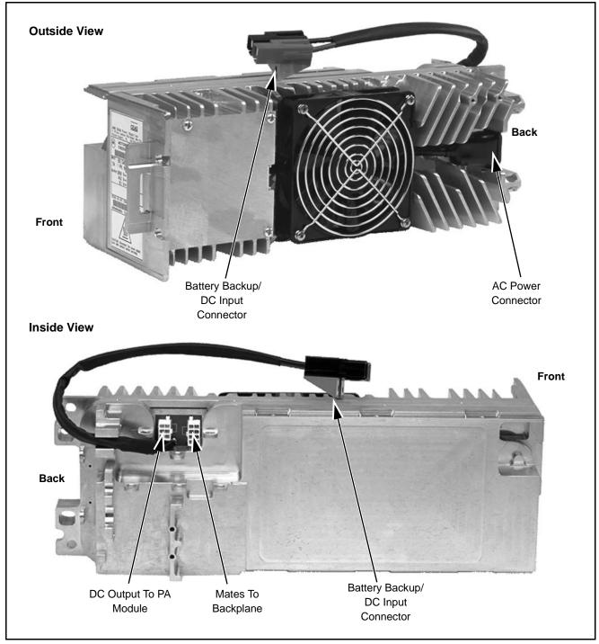
Figure 1. Model DLN6622 Power Supply Module Input/Output Connections
