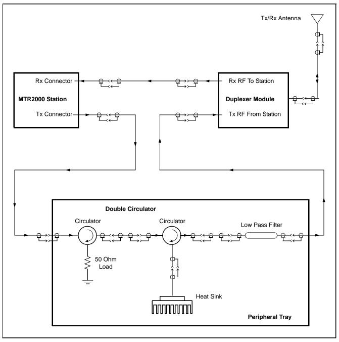
Figure 5. Typical Duplexer Interconnect Diagram
