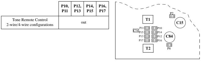
Figure 6. CLN1203 Wireline Interface Board Jumper Settings
