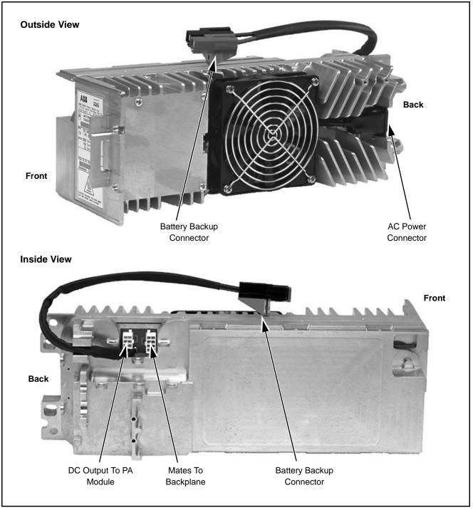
Figure 1. Model CLN1220/DLN6458 Power Supply Module Input/Output Connections
