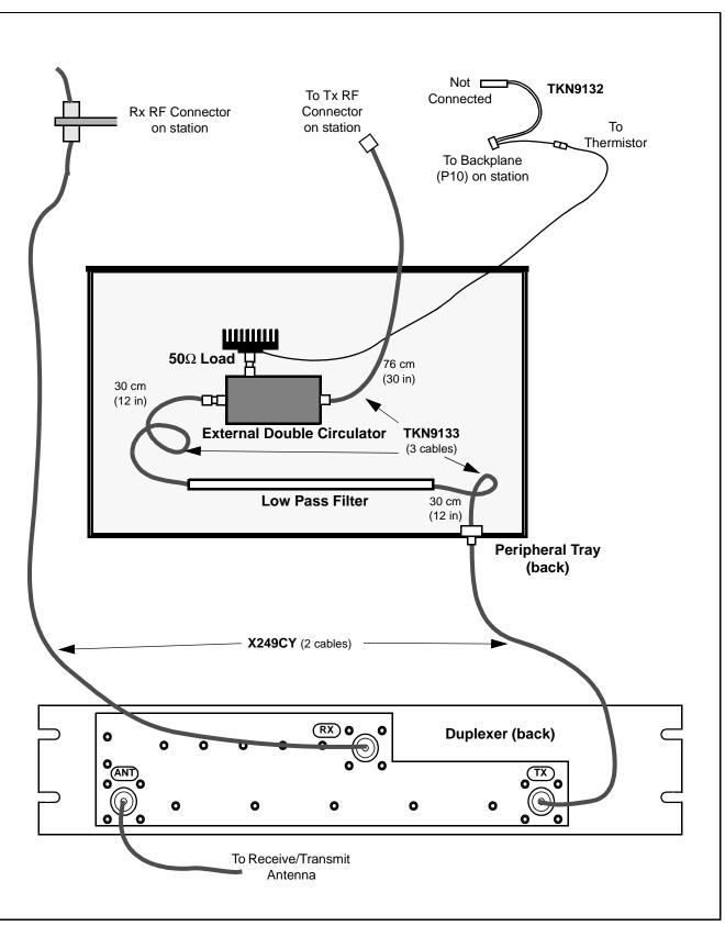
Figure 4. Duplexer and External Double Circulator- Cable Kits
