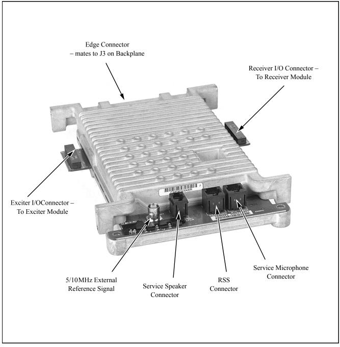
Figure 1. Station Control Module Indicators and Input/Output Connections
