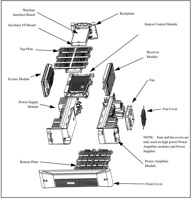
Figure 2. MTR2000 Station Components
