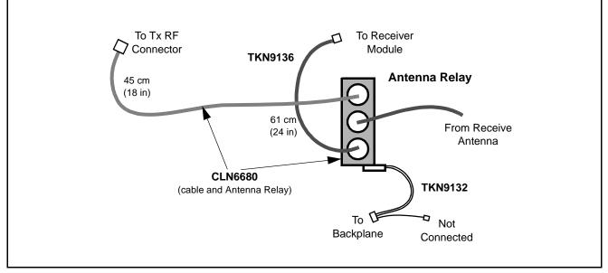
Figure 2. Antenna Relay Only – Cable Kits
