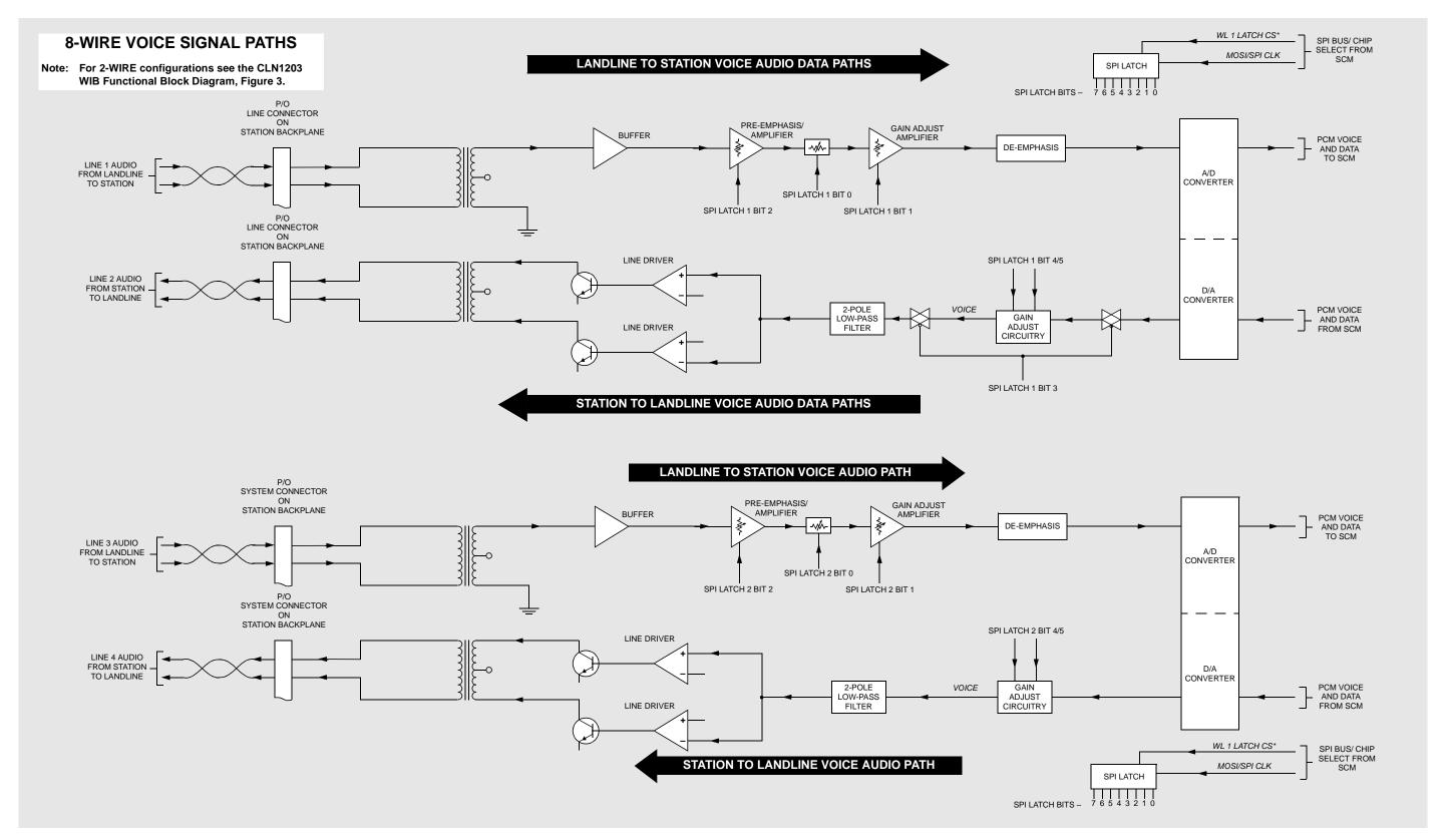
Figure 2. CLN1205 8-Wire Voice Audio Data Path Functional Block Diagram
