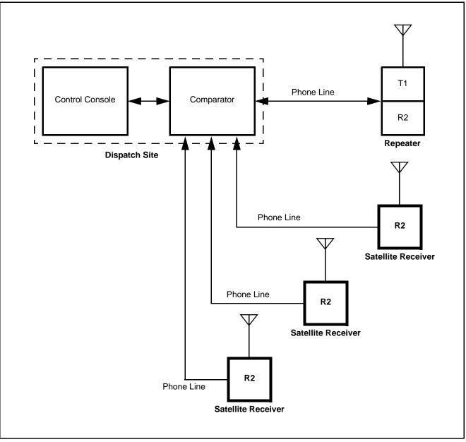
Figure 3. Satellite Receiver Connections Within a Voting System
