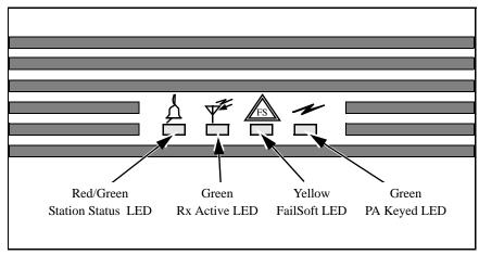
Figure 1. Front Panel LEDs
