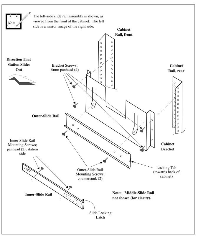
Figure 4. Slide Rail Installation; Option X968AA (Left Side Shown)
