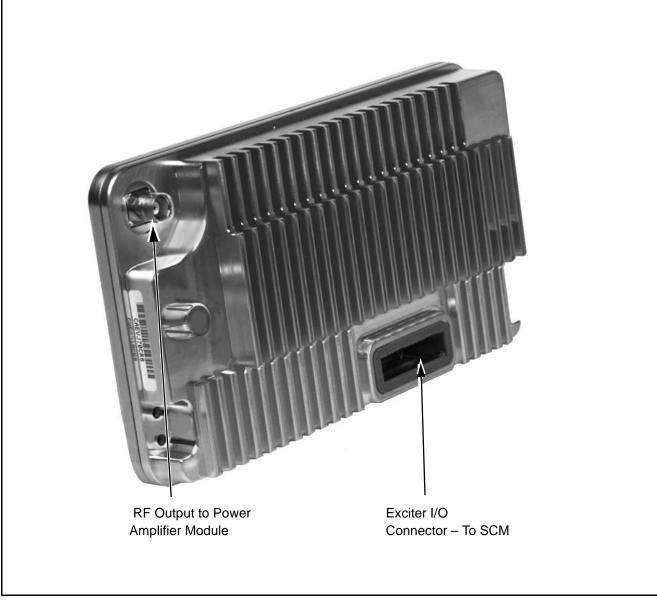
Figure 1. 800/900MHz Exciter Module Input/Output
