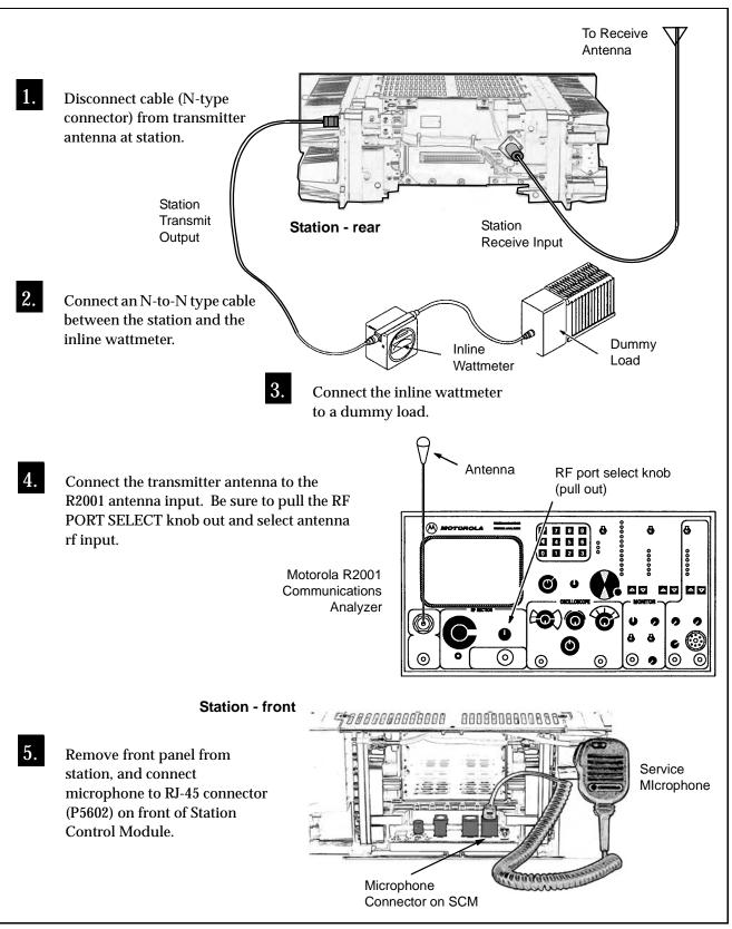
Figure 6. Test Equipment Setup for Verifying Transmitter Circuitry
