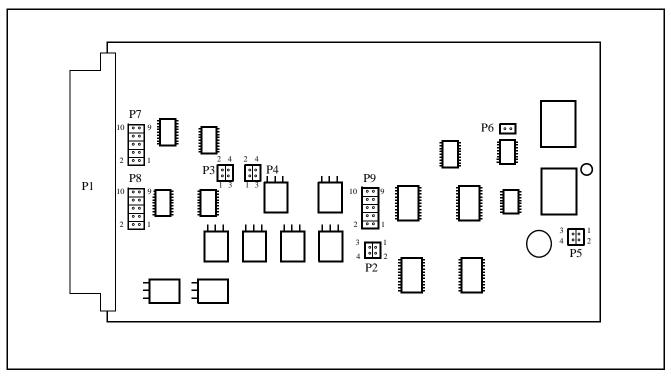
Figure 8. CLN1206 Auxiliary I/O Board Jumpers
