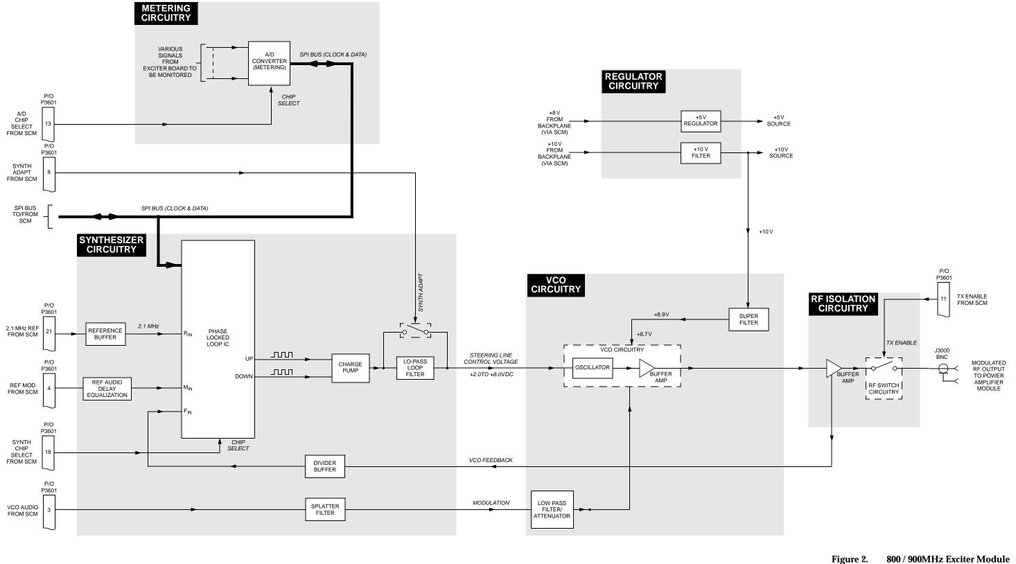
800 / 900MHz Exciter Module Functional Block Diagram
