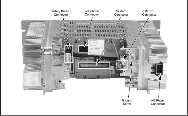
Figure 2. Satellite Receiver Input/Output Connections
