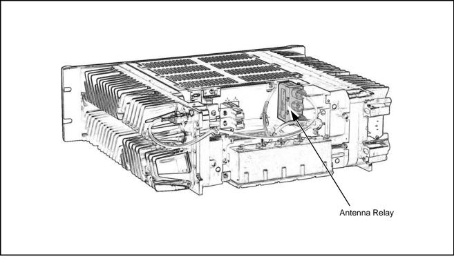
Figure 6. Mounting Position for Antenna Relay Module
