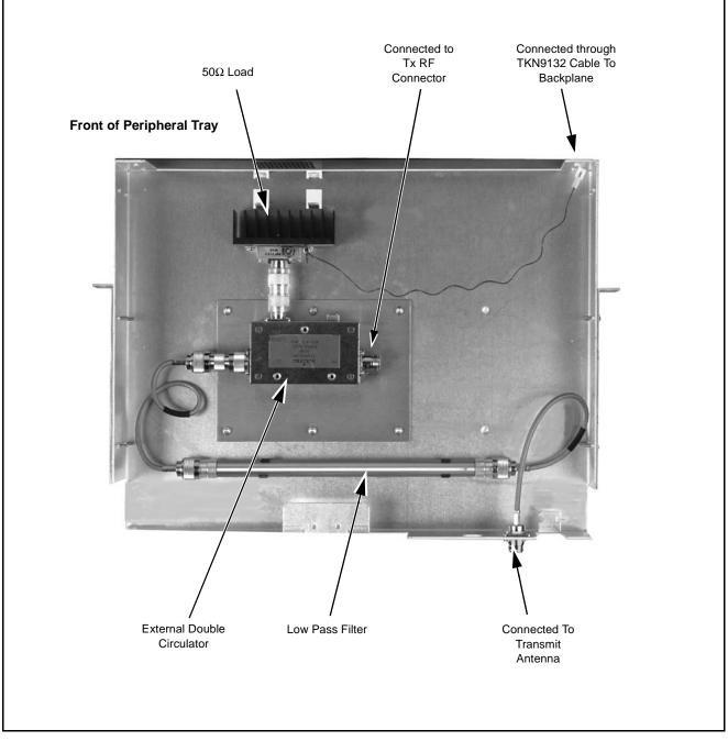
Figure 1. 800/900MHz External Double Circulator Mounted in Peripheral Tray – Inputs/Outputs
