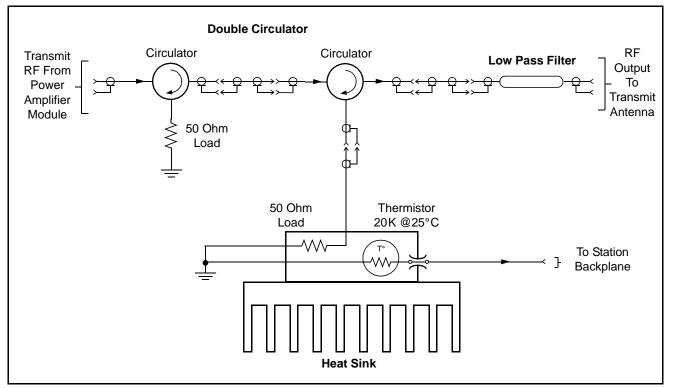
Figure 3. Functional Block and Interconnect Diagram for External Double Circulator Module
