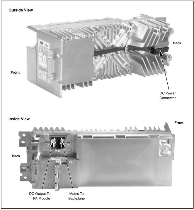
Figure 1. Model CLN1222 Power Supply Module Input/Output Connections
