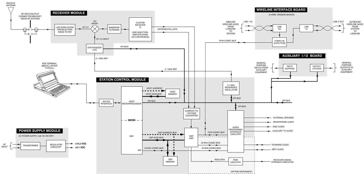
Figure 5. MTR2000 Satellite Receiver **Functional Block Diagram**
