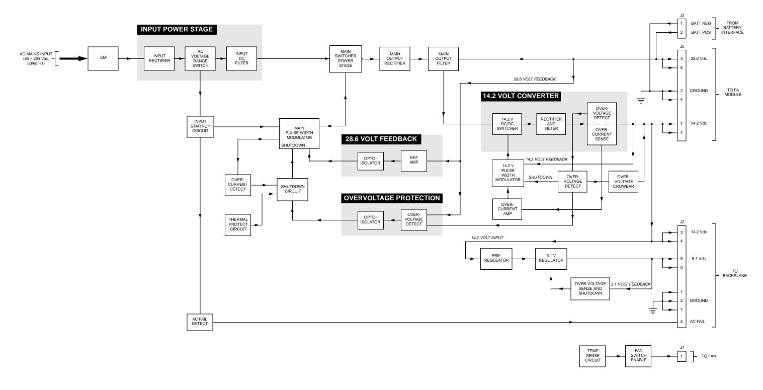
Figure 2. CLN1220/DLN6458 – 500 W Power Supply Functional Block Diagram
