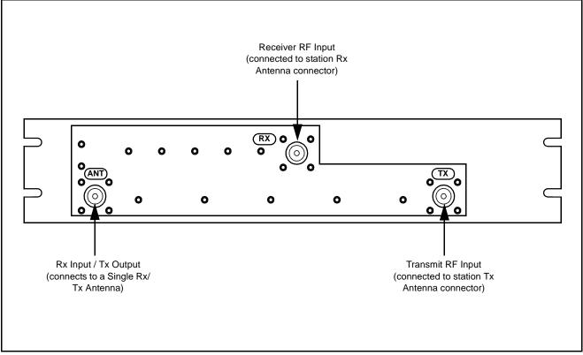
Figure 2. 800/900MHz Duplexer Module – Input/Output Connectors
