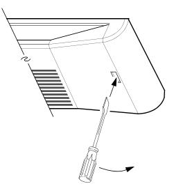
Figure 1. Front Panel Removal
