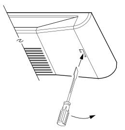
Figure 3. Front Panel Removal
