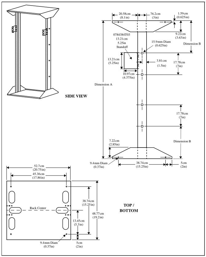
Figure 2. Modular Rack – Dimensions and Clearances
