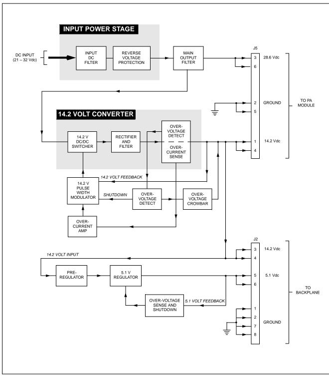
Figure 2. CLN1222 – 500 W DC-Only Power Supply Functional Block Diagram
